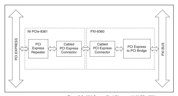
Figure 3-2. MXI-Express Block Diagram with NI PCIe-8361
